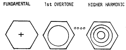
Fig. 11 Modes of the [SS] symmetry class.
